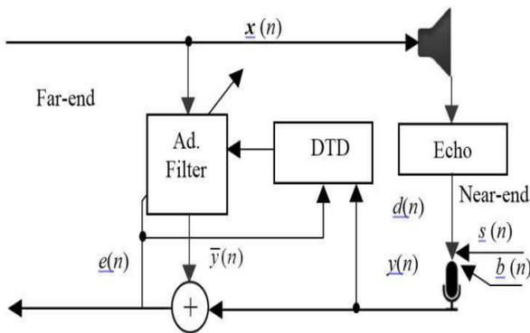
Figure 4: Basic block diagram of AEC with DTD.
