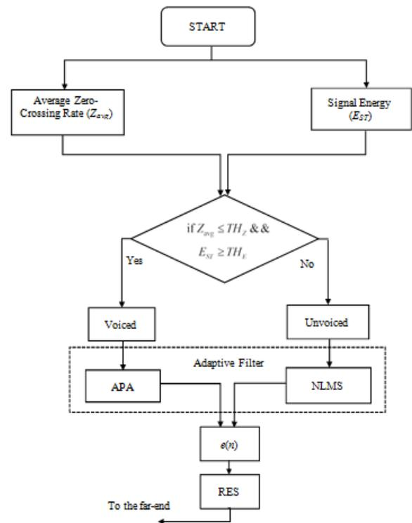
Figure 6: Flowchart of switching AEC
