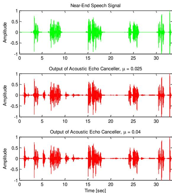
Figure 11: Time-domain speech signals output : for near-end speech signal, acoustic echo canceller for  $\mu=0.025$  and acoustic echo canceller for  $\mu=0.04$
