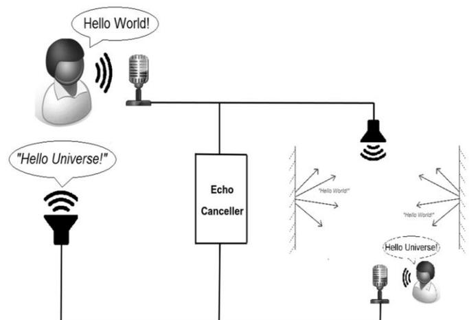
Figure 1: A basic block diagram of acoustic echo with canceller.
