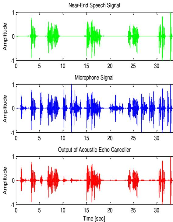
Figure 10: Time-domain speech signals: for near-end speech signal, for microphone signal and output of acoustic echo canceller
