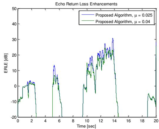
Figure 12: Echo return loss enhancement V/s Time plot for proposed algorithm (for  $\mu=0.025$  and  $\mu=0.04$ )
