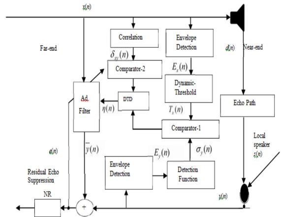
Figure 5: The block diagram of the proposed DTD algorithm.
